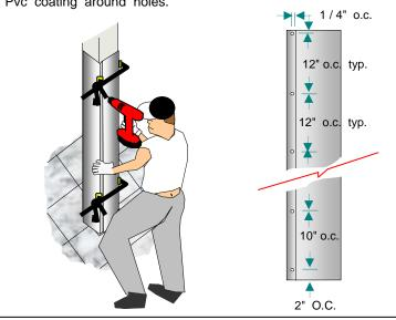
**STEP # 5** Use s.s. pop rivets provided, remove clamps.
