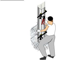
**STEP # 6** use a utility knife to cut pvc coating @ the seam, then peel.
