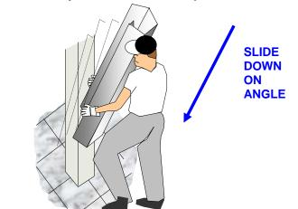
**STEP # 3** start with the top seam, place a putty knife under the 1" overlap, then start to close column with a squeeze clamp or tie straps provided.
